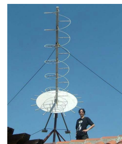
Figure 1: Helix antenna in communications
