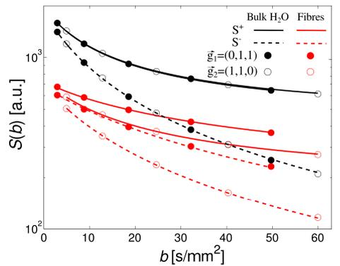
**Figure 2.**  $S^+$  (solid lines) and  $S^-$  (dashed lines) signals from the DW-DESS sequence for two field gradient directions (filled and empty circles) and two ROIs, one in the bulk water (black) and the other in the fibres (red).
