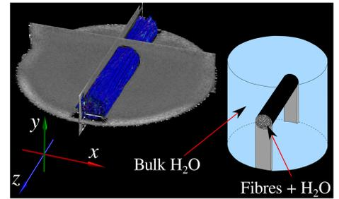
**Figure 1.** Right: schematic representation of the anisotropic diffusion fibre phantom; left: fibre tractography based on the DTI analysis from the DW-DESS pulse sequence, obtained with the help of the ExploreDTI toolkit [9].
