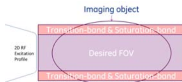
Figure 2. A pictorial demonstration of the walking saturation with 2D excitation. The spins under the transition-bands of the 2D RF are pre-saturated, which otherwise would be excited by the transition bands and wrap-around in to the desired receiving FOV.
