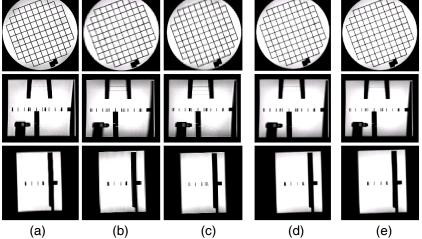
Fig. 1: Super-resolution reconstruction of the ACR phantom from three orthogonal scans; (a)-(c): axial, coronal, and sagittal scans of the ACR phantom (1x1x3mm resolution), (d) image obtained from wavelet fusion (1mm isotropic resolution), and (e) image obtained from image-based super-resolution reconstruction.
