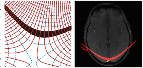
**Fig. 1:** Isocontours of an ExLoc slice selection field (blue), the corresponding encoding field (red) and a cross-section of the selected slice (black)
