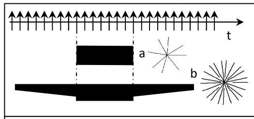
Figure 1. The scheme of golden ratio profile order generate (a) approximately uniform k-space and (b) allows sliding window reconstruction.
