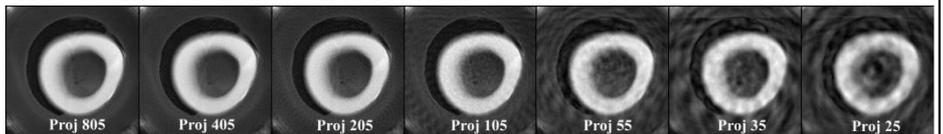
Figure 3. Images of mature bovine tibial mid-shafts reconstructed from fullsampling (805 projections) and undersampling(405,205,105,55,35,25projections) data.
