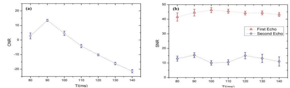
Figure 2. (a)TI versus CNR between cortical bone and muscle. (b)TI versus SNR of cortical bone for dual echos. Error bars indicate standard deviations.
