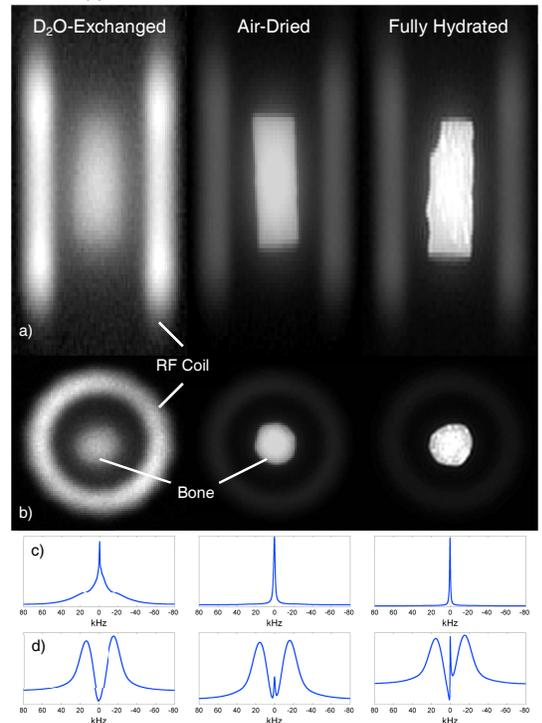
Fig. 3: Sagittal (a) and axial (b) views of D<sub>2</sub>O-exchanged, air-dried, and fully H<sub>2</sub>O-hydrated bone specimens, with corresponding pulse-acquire (c) and IP-DQF (d) spectra. Signal from the cylindrical plastic RF coil support is visible.
