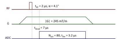
Fig. 2: 3D radial zero echo time (ZTE) pulse sequence with parameters used.
