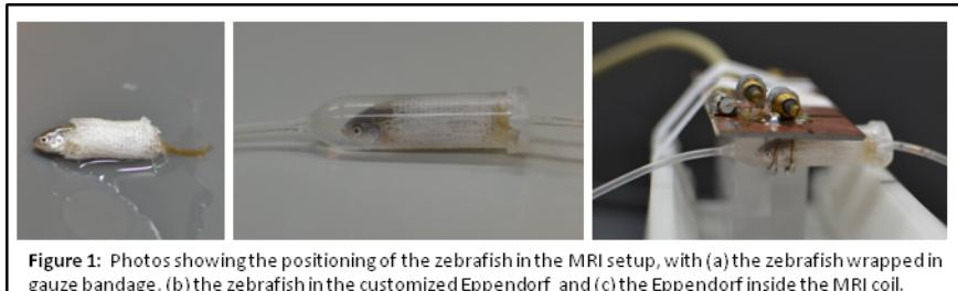
Figure 1: Photos showing the positioning of the zebrafish in the MRI setup, with (a) the zebrafish wrapped in a gauze bandage, (b) the zebrafish in the customized Eppendorf and (c) the Eppendorf inside the MRI coil.
