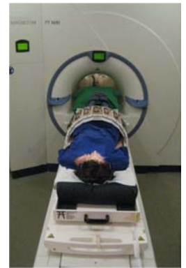
Figure 1: Examinations were performed with a manually positionable AngioSURF table. The custom-built 16-ch coil was positioned around the table with 5 elements below and 11 elements above the
