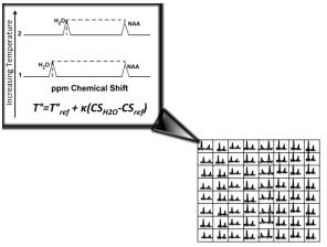
Fig.1 Schematic representation of chemical shift thermometry; an 8x8 multivoxel grid was prescribed for both standard and semiLASER CSI. Temperature is derived from temperature-dependent fluctuations in the water proton chemical shift (CS) compared with the stationary resonance of neuronal NAA
