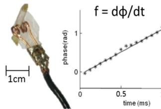
Figure 1: A small field probe (left), was used to independently measure the frequency by fast pulse-acquire readout and a linear fit to the phase (right) to assess the magnetic field drift over time during other sequences.
