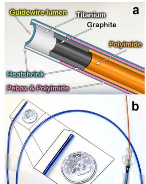
**Figure 1.** Catheter assembly with the susceptibility device. **a:** 3D model of the assembly. **b:** actual catheter picture.
