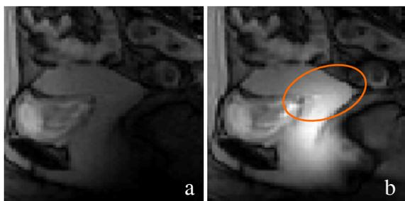
Fig. 1. The signal images from the SNR measurements without (a) and with (b) the internal antenna. In orange the region is shown where the SNR was determined. It is clear that the internal antenna contributes in a great manner to the SNR. Scan duration = 53.7 s;  $T_R = 15$ ms;  $T_E = 1.49$ ms; resolution =  $2 \times 2$  mm<sup>2</sup>.
