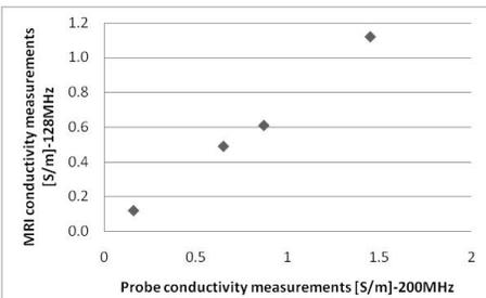
Figure 3. Dielectric probe vs. MRI conductivity data
