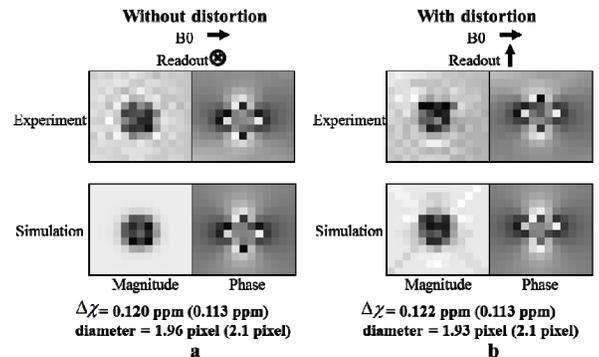
FIG. 2. Phantom studies for susceptibility and diameter measurement. The vessel tube was perpendicular to the main magnetic field and the readout direction was parallel (a) and perpendicular (b) to the vessel tube. All images represent a cross section of the vessel. The calculated  $\Delta\chi$  and diameter shown on the bottom of each figure were within 10% error of the known values given within the parentheses. One pixel size is .47x.47 mm<sup>2</sup>.
