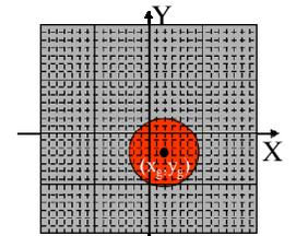
FIG. 1. Diagram representing relative locations of MR pixels (solid lines), a cross-sectional view of vein of interest (red circle), and sub-pixel gridding lines (dashed lines).
