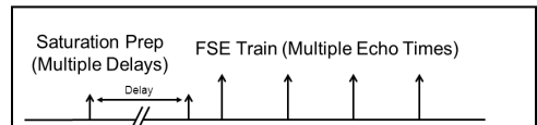
Figure 1. By running a saturation recovery FSE with multiple delay and spin echo times, QMAP acquires contrasts necessary for T1 and T2 relaxation time and proton density mapping.
