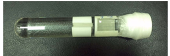
Figure 1 Crossing fibre phantom immersed in cyclohexane. The layers are squeezed between two plastic rods.
