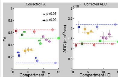
Figure 3: FA and tADC values for each compartment, corrected for SNR and temperature. Colors indicate similar capillary i.d., while symbols indicate radial position.
