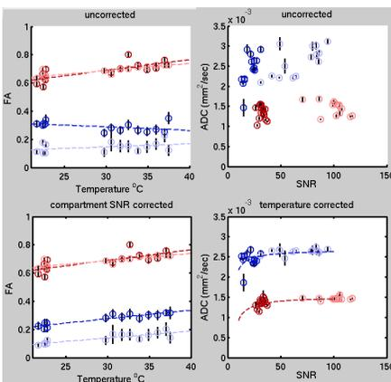
Figure 2: Representative FA and tADC data, before corrections for temperature and SNR, for four compartments (red/pink = 20  $\mu\text{m}$  i.d. capillaries; blue/cyan = 200  $\mu\text{m}$  i.d.), with regression fits.
