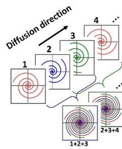
**Fig. 1** An example of shifted interleaved acquisition for VDS DTI. The numbers and colors denote diffusion directions
