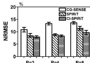
**Fig. 4** Mean NRMSE of reconstructed DW images in all directions using three methods
