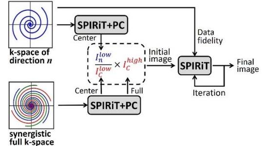
**Fig. 2** CI-SPIRiT. 1) SPIRiT and Phase correction (PC); 2) IRCR using low resolution images  $I_n^{low}$  and  $I_c^{low}$  from k-space center and high resolution image  $I_c^{high}$ , where 'c' denotes synergistic k-space. 3) Iterative reconstruction using SPIRiT.
