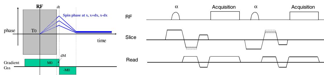
**Figure 2 (right):** Inverted slice select generates +/- flow encoding, dotted lines show timing correction implemented as a change to G2 amplitude.
