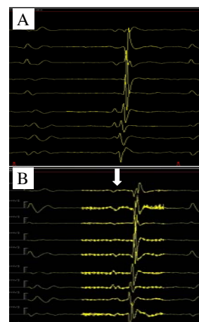
Figure 2: examples of two EP signals (1 cardiac cycle) collected during T1w delay enhanced (A) and balanced-SSFP (B) sequences. The white arrow in (B) shows the artefact on EP signal due to gradient switching. The callipers on the left side of (B) correspond to 1 mV amplitude.
