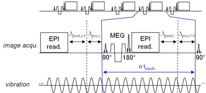
**Fig.1:** Sequence timing diagram illustrating the delay of single shot image acquisition relative to continuously applied harmonic vibrations in order to achieve the dynamic capture of wave propagation.
