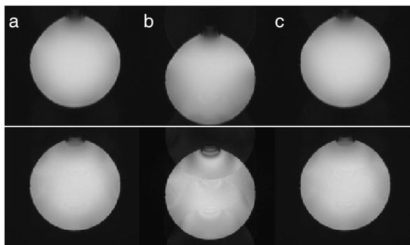
**Fig. 1:** An isocentric slice in a phantom acquired with partial Fourier (upper) and GRAPPA (lower). In (a) the MR system frequency was correctly adjusted, in (b) and (c) it was shifted by  $-200$  Hz. (b) was obtained without, (c) with correspondingly adapted ADC settings, i.e. a frequency offset for all echoes and a phase linearly modulated along the echo train. The apparent phantom shift in (b) is due to the linear phase evolving along the echo train which is corrected for in (c).
