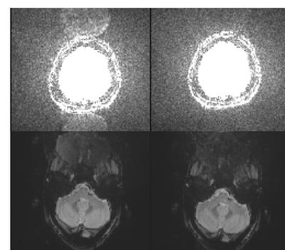
**Fig. 3:** In vivo examples with the MR system frequency adjusted to the full stack of slices. Residual ghosting occurs in upper and lower slices (left). It is reduced when using a slice-specific frequency setting for the data acquisition, i.e. frequency and phase settings for the ADC.
