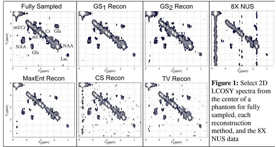
**Figure 1:** Select 2D LCOSY spectra from the center of a phantom for fully sampled, each reconstruction method, and the 8X NUS data
