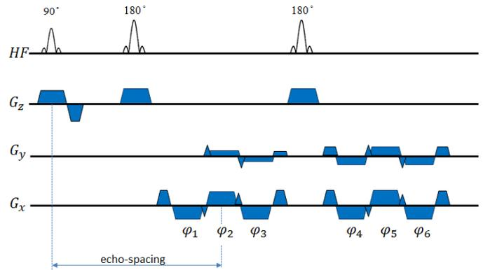
Fig. 1. Sequence diagram of radial GRASE. To acquire different k-space views (i.e. to alter the angle between two subsequent views), blipped gradients in x- and y- direction were used.
