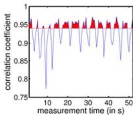
**Fig. 2.** The first 50 s of the generated trigger signal are shown. The threshold at a correlation coefficient from 0.94 is delineated by a red line which defines the red marked breathing phase.
