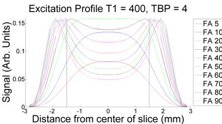
Figure 2. Excitation Profile for TR=20, T1 = 400, TBP=4
