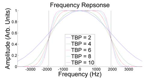
Figure 1. Frequency response to Hamming windowed sinc pulse with different TBP.
