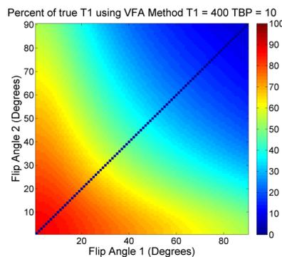
Figure 6. Percent of true T1 for different combinations of flip angle TBP 10, T1<sub>true</sub>=400
