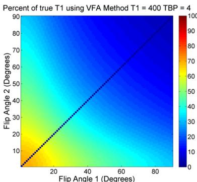
Figure 5. Percent of true T1 for different combinations of flip angle TBP 4, T1<sub>true</sub>=400
