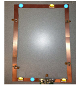
Figure 1: Surface coil (23cmx15cm) with Vitamin E markers (yellow) and fluorine markers (blue)
