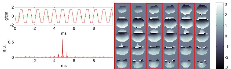
**Fig.3.** SCOPE 3D pulse design example. Left: spokes pulse with 23 spokes. Right: excitation phase through Bloch simulations (in red columns) compared to design template.
