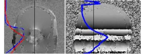
**Fig 1.** 1D SCOPE phase modulation. Left: unwrapped phase from calibration scan with a line profile (blue), along with its low-pass filtered version in red) used for pulse design. Right: excitation phase and a line profile (unwrapped).
