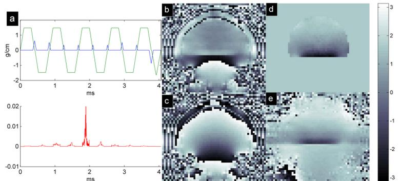
**Fig.2.** 2D SCOPE pulse design example. (a) gradient and RF waveforms using 9 spokes; phase images at echo time using SCOPE 2D pulse (b) and a regular sinc pulse (c); (d) shows the phase map used in designing the pulse in (a); and (e) shows the phase difference between (b) and (c).
