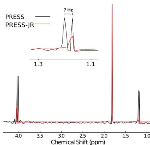
Figure 2: Spectra of acetate and lactate at 100 ms for PRESS (above) and PRESS-JR with 3 refocusing units.
