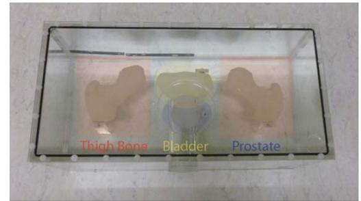
**Figure 1:** Phantom setup. Components that mimic left and right thigh bone (red), bladder (yellow), and prostate (blue) are fixed inside a water-filled glass box. An endorectal coil can be mounted under the prostate
