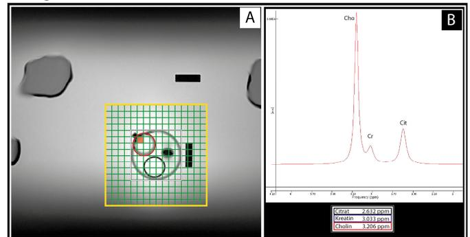
**Figure 2:** <sup>1</sup>H MR spectroscopic imaging (2D-PRESS) of the MR-PET phantom at 3 T. (A) Field-of-view of SI across the “prostate” (grey circle) filled with a model solution of choline (100mM), creatine (50mM), and citrate (200mM). Black bars: Fixation of phantom components. (B) <sup>1</sup>H MR spectrum from voxel (red) inside the “prostate” with resolved resonances.
