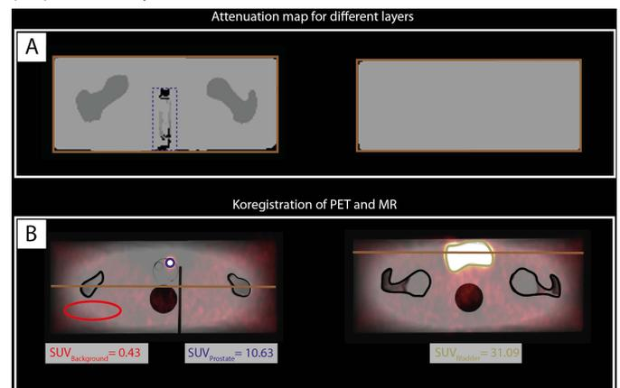
**Figure 3:** (A) Attenuation-map reconstruction (coronal slices for “thigh bones”, right, and “bladder”, left). (B) Overlays of transversal MR-PET scans. “Thigh bones” were correctly registered as fat signal (dark grey). As required, “bladder” is not distinguished from background signal. The air-filled endorectal coil is marked (A, blue). <sup>68</sup>Ga solution was added to the content of “bladder” (yellow), “prostate” (blue) and glass box (red). Measured SUV values are indicated.
