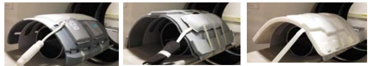
Fig. 1: 16-CH conventional AA coil (left), 16-CH PET/MR prototype AA1 coil (middle) and 16-CH improved PET/MR prototype AA2 coil
