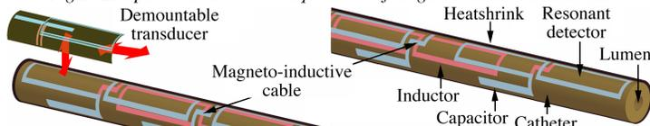
Fig. 2: Integration of thin-film circuit on catheter.
