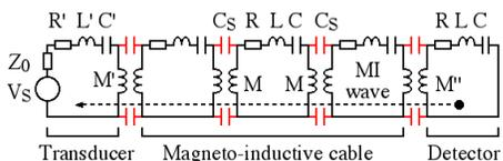
Fig. 1: Lumped-element circuit equivalent of magneto-inductive receiver.
