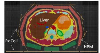
Figure 1. Schematic diagram of the arrangement of HPM, receive coils, and the human body.
