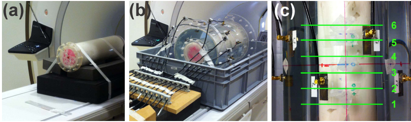
Fig. 1 (a) H&N phantom in bore alone (setup 1) (b) H&N phantom in MRlabcollar (setup 2). Here the phantom is in the same orientation and position as from setup 1 (c) Top view of phantom in setup 2 showing approximate slice locations for the primary region of interest.
