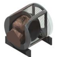
Figure 3. Helmet array coil positioned inside 30 cm NMR transmit coil.
