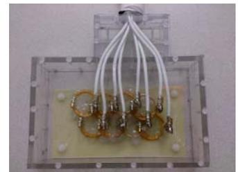
Figure 2: 8-channel array using integrated balun coils.
