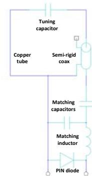
Figure 1: IBC schematic.
