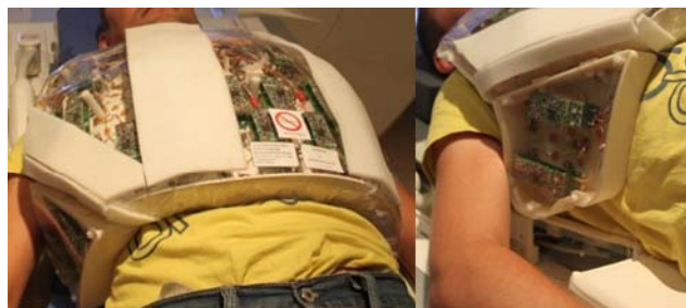
Fig.1 New 64-channel cardiac coil. The chest part can be closely matched to the thorax with a hinge for improved accelerated imaging.
