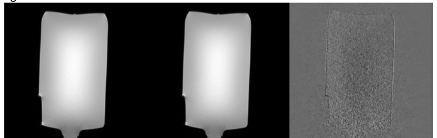
Fig. 3. MPRAGE images of a cylindrical phantom. Left to right: surface scanner off/out-bore, on/in-bore, difference of the first two images (normalized scale as the original scale)
