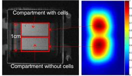
**Figure 3**: Left: Proton image of the 3<sup>D</sup>-KITChip within the bioreactor. Right: Corresponding <sup>23</sup>Na – CSI signal of the two compartments.
