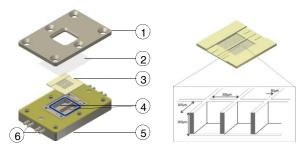
**Figure 1**: Left: Exploded view of a 3<sup>D</sup>-KITChip-containing MRI-compatible bioreactor. 1=upper lid, 2=microscope cover slip, 3=3<sup>D</sup>-KITChip, 4=independently perfused compartments, 5=bioreactor housing, 6=connection for perfusion.
