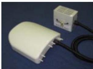
**Figure 1** – <sup>13</sup>C/<sup>1</sup>H liver coil built for in vivo human <sup>1</sup>H decoupled <sup>13</sup>C spectroscopy
