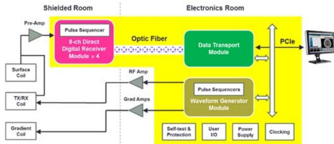
**Figure 1:** Block diagram of the distributed multichannel MRI console
