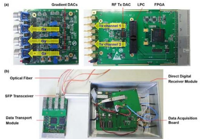
**Figure 2:** Photos of (a) a waveform generation module and (b) a direct digital receiver module in a basic 4-channel configuration linked to a data transport module over an optical fiber pair.
