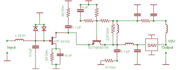
**Fig. 1.** Preamplifier modified to include SAW filter.
