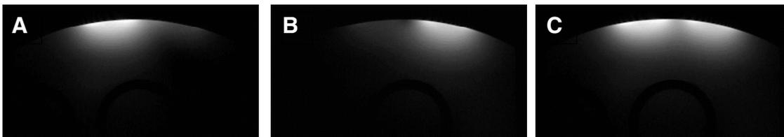
**Figure 4.** Images from 2 coil system **A, B** individual coils images and **C** sum of squares image
