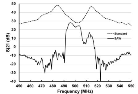
**Fig. 3.** Output characteristic of preamplifier with integrated SAW filter when connected to noise matched receive coil.
