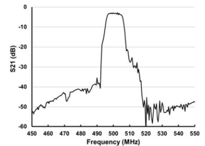
**Fig. 2.** SAW filter transfer characteristic.
