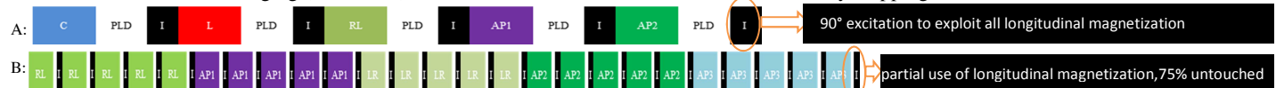
Figure 1: A) standard VS-ASL with multi slice read-out and B) VS-DASL with small flip angle single shot TFEPI: labeling efficiency is varied in different directions such as anterior-posterior (AP) and right-left(RL); imaging is represented by (I)
