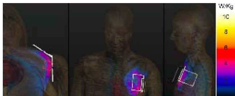
Fig 3. 10-g avg SAR, 120 MHz, 1 W per channel. 8
