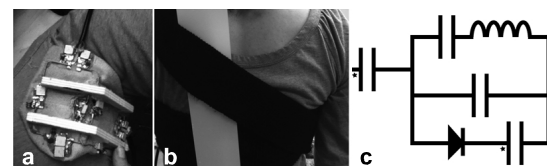
Fig. 1 Quadrature coil used for ^{31}\text{P} transmit/receive of and ^1\text{H} receive (a). Radiative element on back (b) provides majority of ^1\text{H} excitation held in place by custom fabric housing. (c) Each loop element contains a modified dual-resonant unit to detune resonance at 300 MHz during transmit (* indicates choke inductor).
