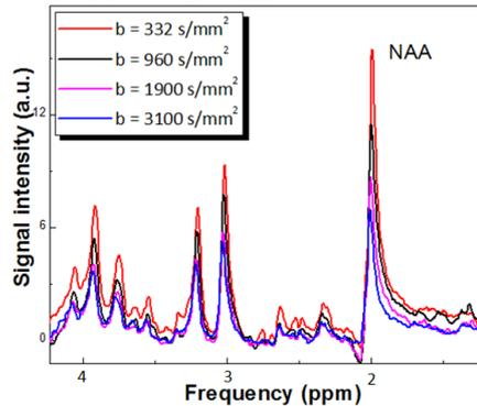
Fig.3: Examples of spectra acquired at different b values for direction (0,0,1). Note the sharp decrease in the NAA peak.
