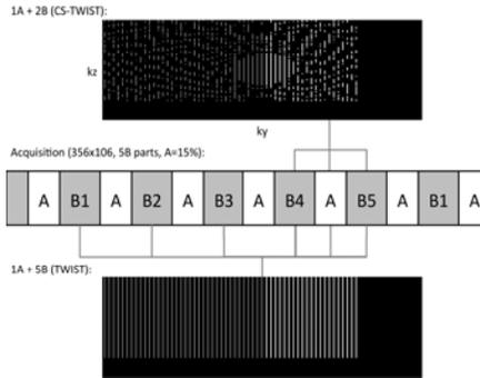
**Figure 1:** View-sharing is reduced from full k-space (TWIST) to its minimum using adjacent acquired parts of k-space only (CS-TWIST). Compressed Sensing allows for the reconstruction of images for CS-TWIST.
