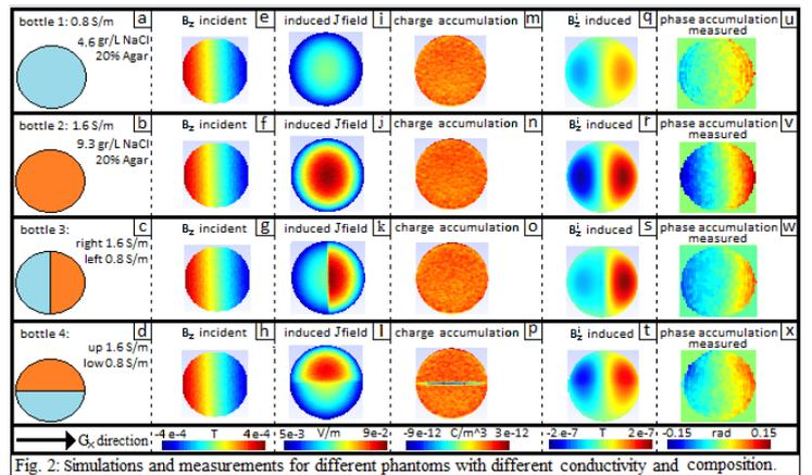
Fig. 2: Simulations and measurements for different phantoms with different conductivity and composition.
