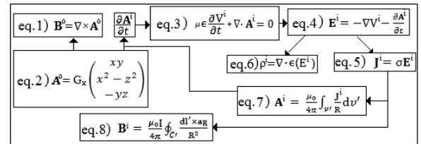
b) Simulation of induced magnetic field  $B$  (Fig. 2q-t): Assuming electrostatic conditions, we derived from the induced eddy-current density the induced vector potential  $A^1$  (eq.7) and magnetic field  $B^1$  (eq.8) through the Biot-Savart law. If needed, higher order q.s. corrections  $A^1$ ,  $B^1$ , and  $E^1$  can be calculated by a new iteration with the updated magnetic vector potential. In our case, we iterated the loop two times, thus including first and second order corrections.
