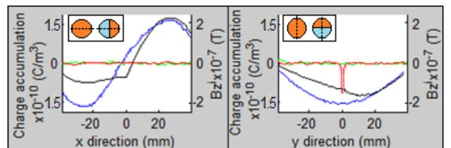
Fig.3: Comparison between the induced  $B_z$  field and the charge accumulation for bottle 2 (blue, green lines respectively) and 3 (black, red lines respectively) on the left, bottle 2 (blue, green lines respectively) and 4 (black, red lines respectively) on the right.
