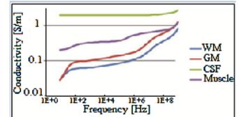
Fig. 1: Conductivity values as a function of the frequency.
