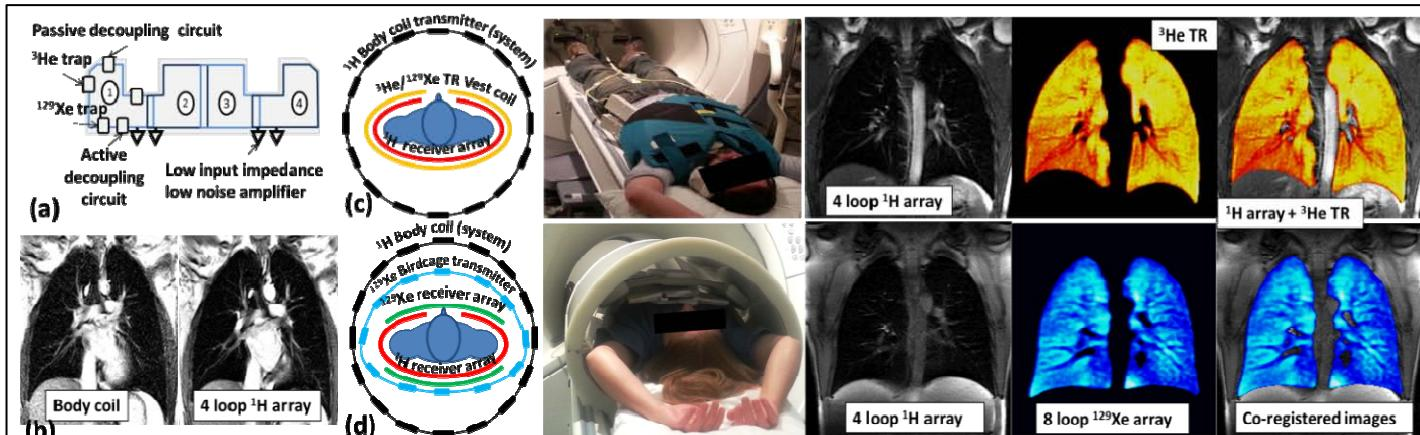
**Figure 1:** (a)  $^1\text{H}$  receiver array design, (b)  $^1\text{H}$  SNR comparison between body coil and receiver array (c)  $^1\text{H}$  receiver array with  $^3\text{He}/^{129}\text{Xe}$  TR vest coil and (d) two birdcage transmitter and two dedicated receiver array for  $^1\text{H}$  and  $^{129}\text{Xe}$
